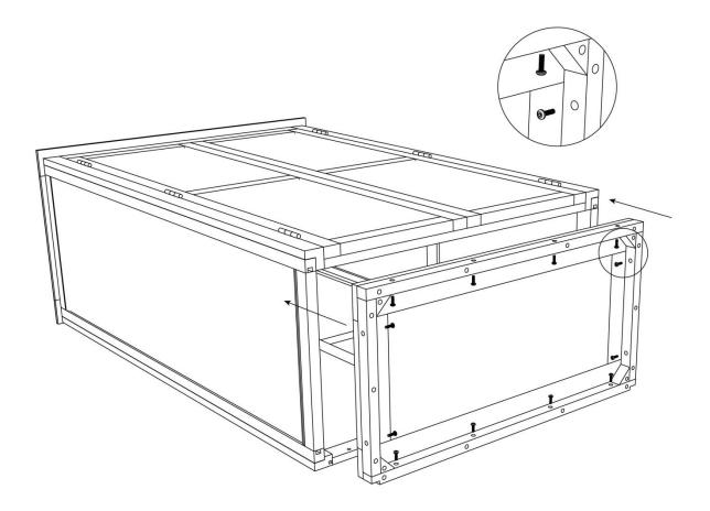
Step 9: Tighten the Allen Bolts properly.
