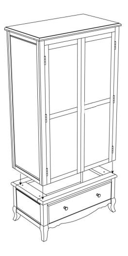
Step 11: Tighten all the 4 Allen Bolts on the corners with Washers using Allen key.
