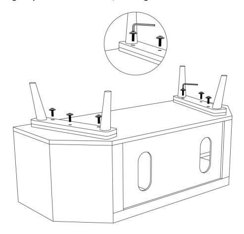
Step 2: Tighten all the Allen Bolts of the Legs properly by using Allen Key.
