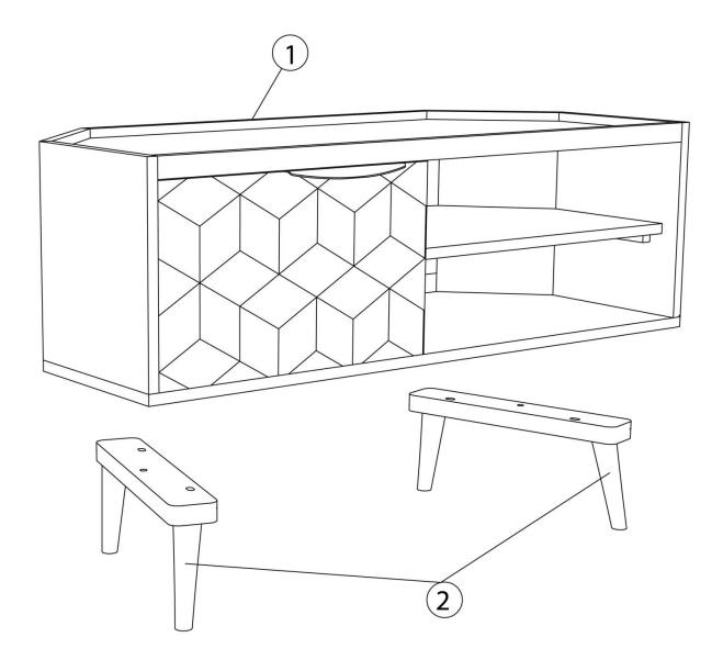
Step 1: Align the legs as per the Slotted holes, and Align the Allen bolts.
