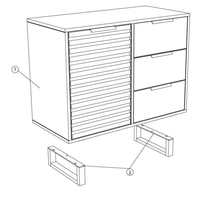
Step 1: Align the legs as per the Slotted holes, and Align the Allen bolts.
