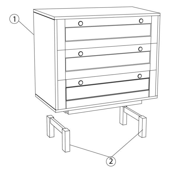
Step 1: Align the legs as per the Slotted holes, and Align the Allen bolts.
