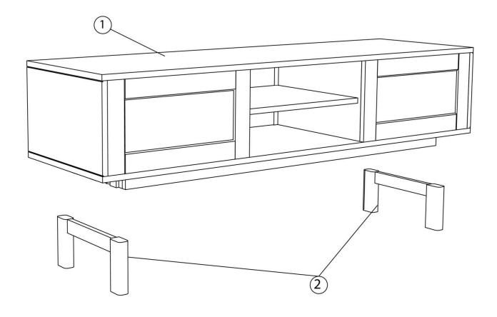
Step 1: Align the legs as per the Slotted holes, and Align the Allen bolts.
