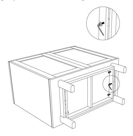
Step 2: Tighten all the Allen Bolts of the Legs properly by using Allen Key.
