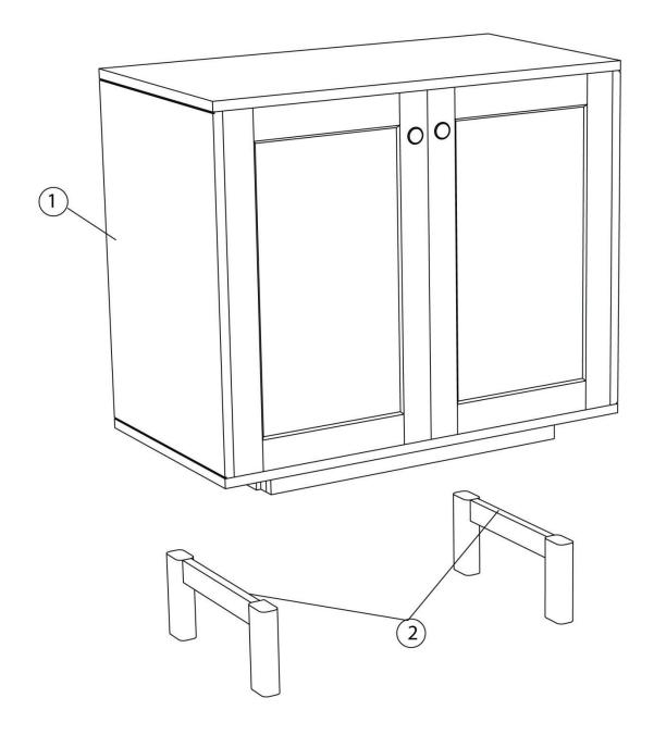
Step 1: Align the legs as per the Slotted holes, and Align the Allen bolts.
