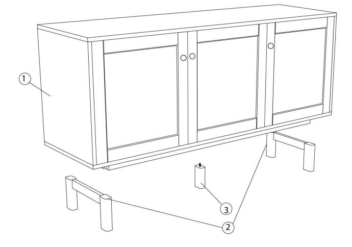
Step 1: Align the legs as per the Slotted holes, and Align the Allen bolts.
