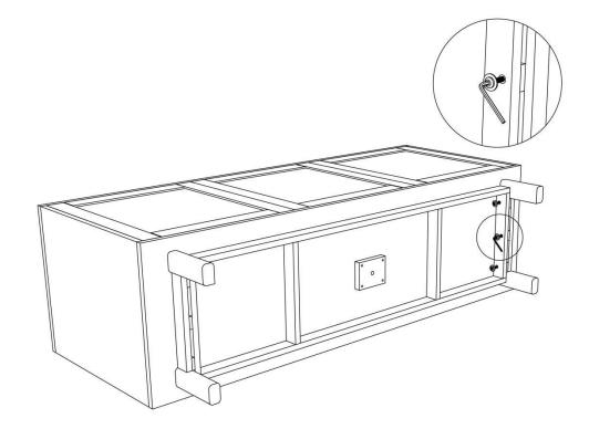
Step 2: Tighten all the Allen Bolts of the Legs properly by using Allen Key
