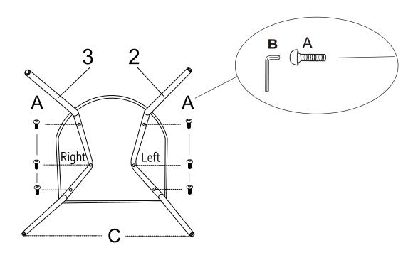
**Step 2**: Use adjustable feet (C) to level the chair on ground.
