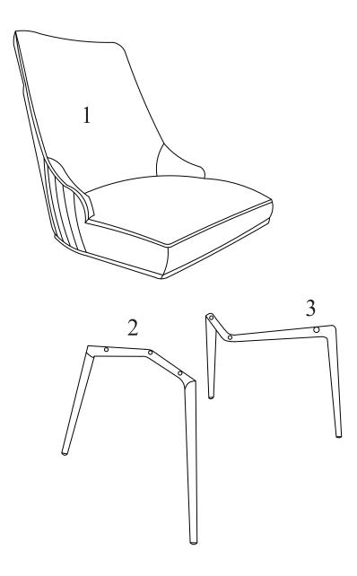
**Step 1**: Attach the seat(1) to the leg frames(2)(3) and fix through holes using bolts(A). Then tighten the bolts using the allen key(B) provided.
