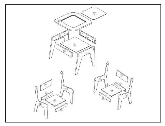
Step 1: Use Screw bolt Ax4pcs and screw nut Bx4pcs to fix slat Part 2x2pcs to side panel Part 1, and put cam lock nut Fx2pcs into the screw holes of side panel Part 1, Put Screw nuts Bx4pcs into the screw holes of slat Part 2x2pcs
