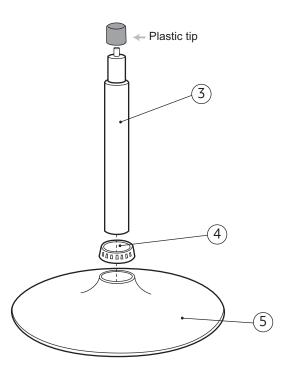
**Step 3:** Position the seat as shown and insert the gaslift (3) into the upper leg (2).
