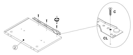
Need to assemble drawer runner in the correct pilot hole as the diagram indicates.
