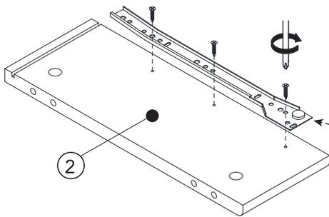
Need to assemble drawer runner in the correct pilot hole as the diagram indicates.
