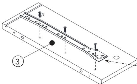
Need to assemble drawer runner in the correct pilot hole as the diagram indicates.
