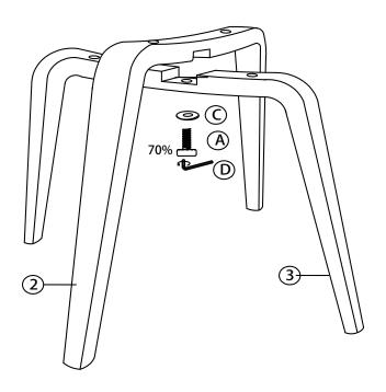
**Step 2:**Attach seat(1) to leg and fix through hole using bolt(B) and flat washer (C). Then tighten all bolts using allen key(D) provided to 100% of the thread
