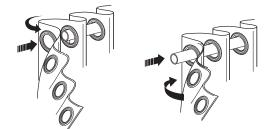
• We advise 3 eyelets at the beginning of the pole, then a bracket, then 2 eyelets in between the next bracket, then the rest of the curtain to the centre bracket.
