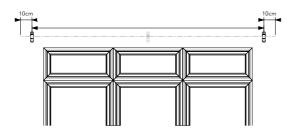
Note: For 120-210cm and 210-360cm model, you may wish to enhance the look and performance of your curtain pole by centralising the joining piece and hiding it behind the centre bracket. To do this follow the steps below.
