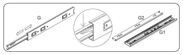
Whilst pushing the leaver down, slide the runners in opposite directions to each other to separate. Please do not wipe off the grease as this will help the runners slide back together at the end of assembly.
