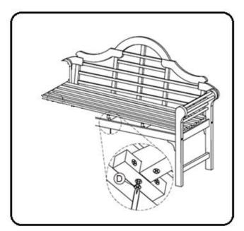
Place the seat on the front bar Loosely secure the seat in place
