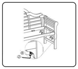
Using part B fix the corner supports to both the front Bar and back rest
