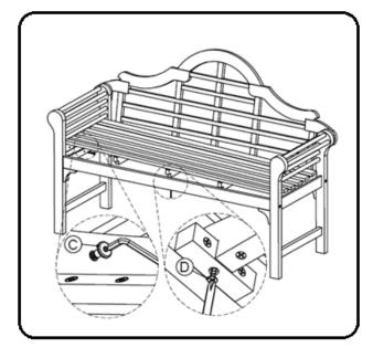
Secure the second arm to the bench. Secure the seat into the arms using Parts C and D.
