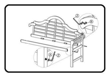
Attach an Arm to the back rest as shown, Add the front bar.
