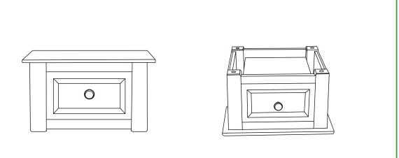
Step1: Turn the A Cabinet upside down onto a clean flat surface.
