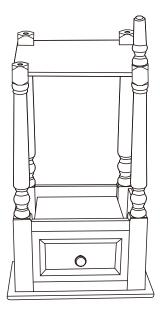
Step 3: Turn the B cane shelf upside down on the 4 long legs to make their 4 holes to fit; then insert D short legs in the the slot of shelf and long legs.
