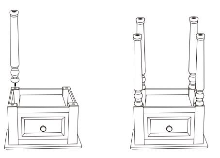
Step 2: Insert one long leg (C) into the slot in the cabinet body as shown. Then repeat the other 3 legs (C) and fully tighten fixings.
